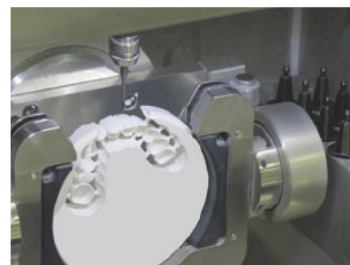
Maximum disk thickness: 35 mm. Maximum milling bur protrusion: 35 mm.
